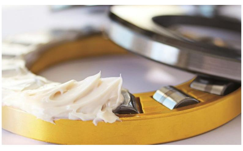
Greases are the best choice if the lubricant is to stay in place at the friction point long term. Not only do they provide good lubrication; they also protect the friction point against external influences like splash water, humidity, contamination and wear..
